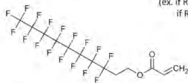
Polyfluorinated polymeric unit (ex. 1H,1H,2H,2H-perfluorodecyl acrylate)
